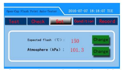
The interface can set is expected to point value and the atmospheric pressure value: click "is expected to flash point" or "high pressure" of the "change", into the expected flash point or pressure setting interface:
