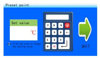
The interface, click the "Settings" regional, above the keyboard is expected to flash point set value input box at the blinking cursor, digital input, and verify input according to the |. To delete a digital input, you can click ".". Click on the right side of the screen "exit" icon, the flash point is expected to exit the setting interface.
