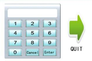
To adjust the date, time, click on the interface above the time display area, the keyboard input box that is to be modified to display (years, months, days, hours, minutes, seconds to show the region to?" Instead, the need to be in the order of one by one, after the number of seconds to enter the digital input, you can click on the "OK" button to complete the change. If you quit, please click Cancel ".
