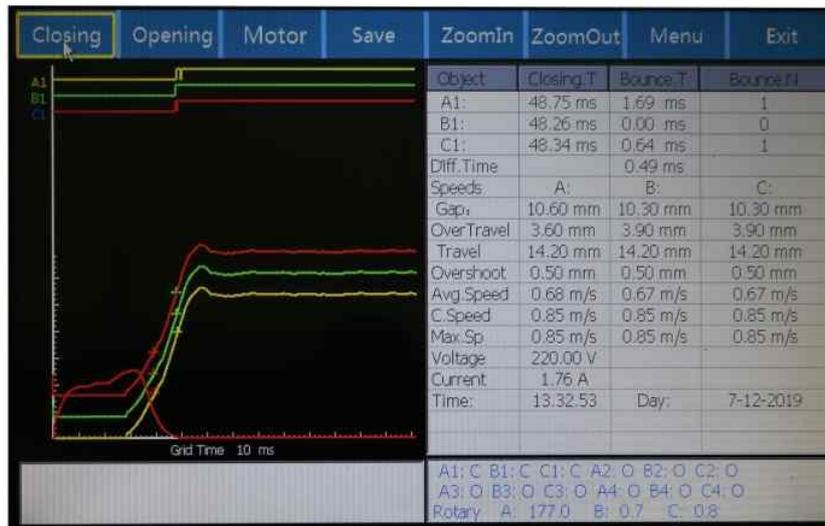
5) The opening test data of the 3-way sensor is shown in the figure below:
