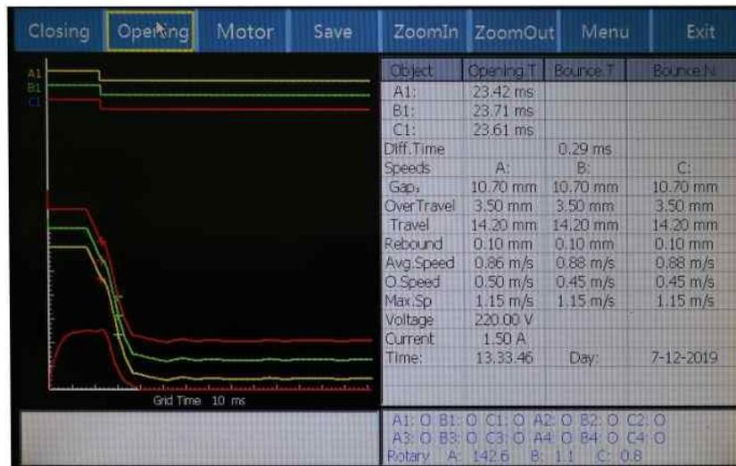
**C. Reclosing test:** First, set the time of C-O, O-C, O-C-O, and then enter the test interface, as shown in the figure below:
