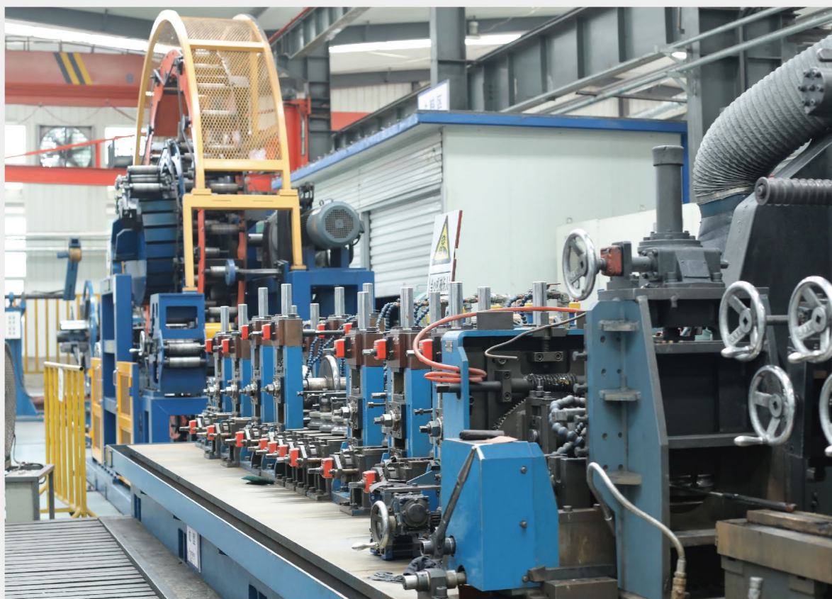
Korean KTM high-frequency welded tubes production line
