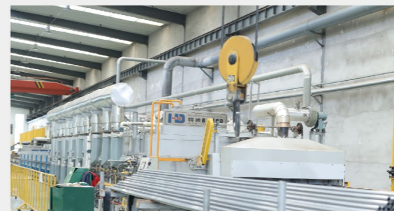
Korean Handuk roller hearth type continuous anaerobic annealing furnace
