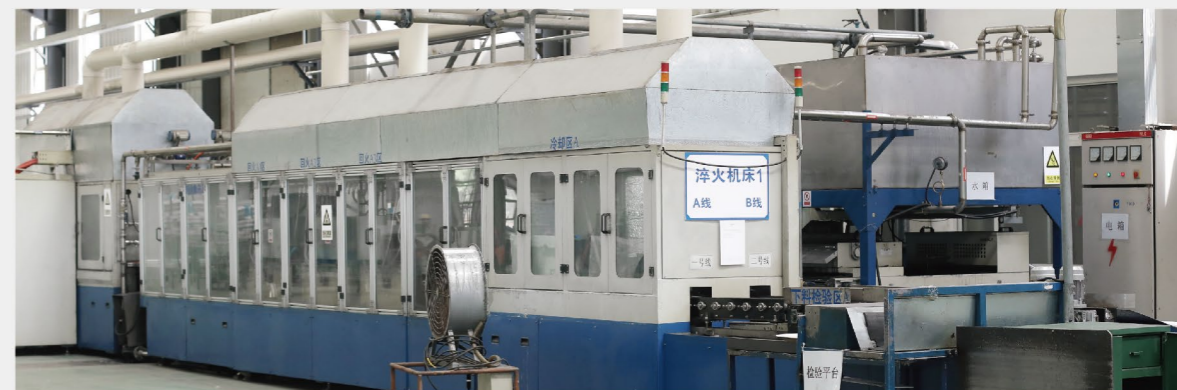
Fully automatic high frequency induction quenching/straightening production line for side door impact beam
